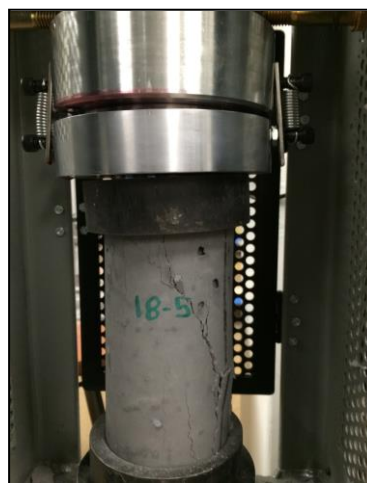
Figure 9: Concrete Compression Test
