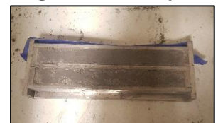
Figure 10: Shrinkage Test Molds
